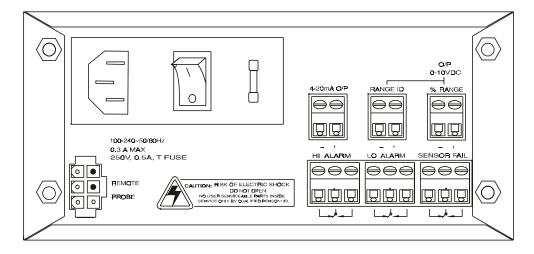
Figure 3-1 Electrical Connectors for AC Control Unit
